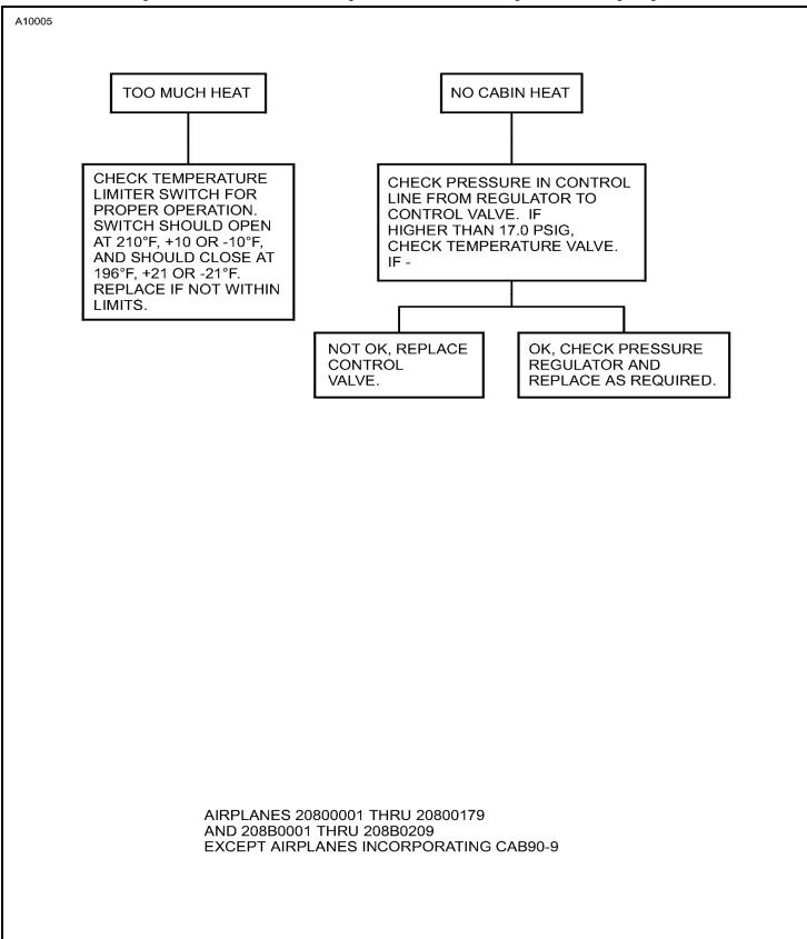
Figure 103 : Sheet 2 : Cabin Heating and Windshield Defrosting Troubleshooting Diagram
