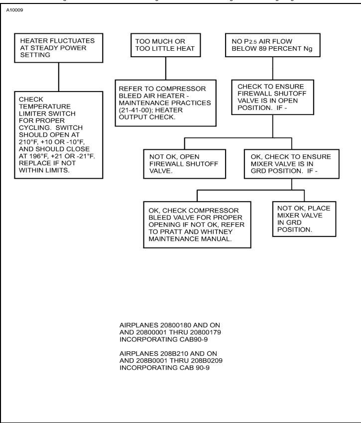
Figure 104 : Sheet 2 : Cabin Heating and Windshield Defrosting Troubleshooting Diagram
