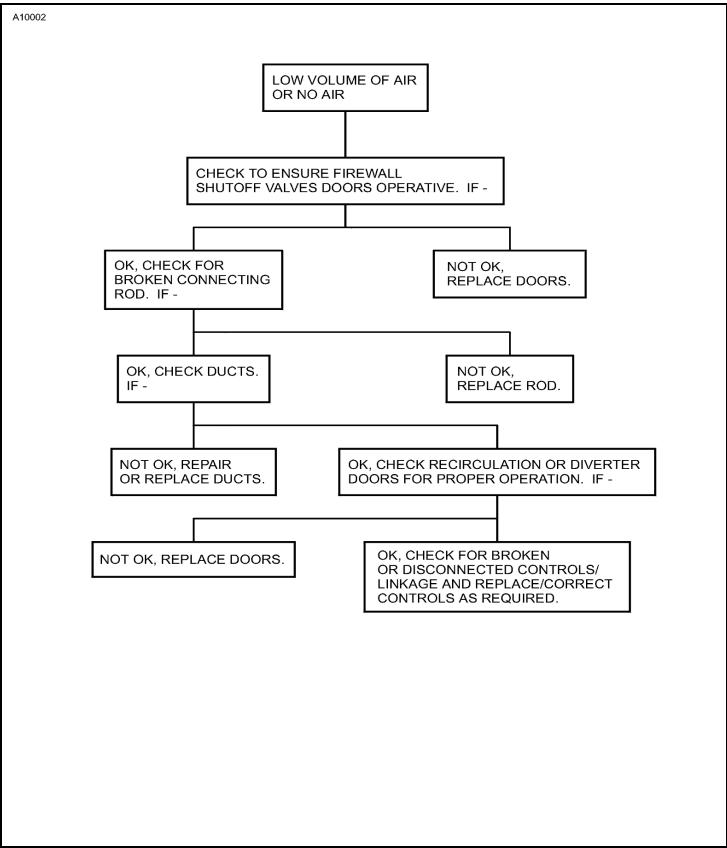
Figure 101 : Sheet 1 : Compressor Bleed Air Heater Troubleshooting Diagram
